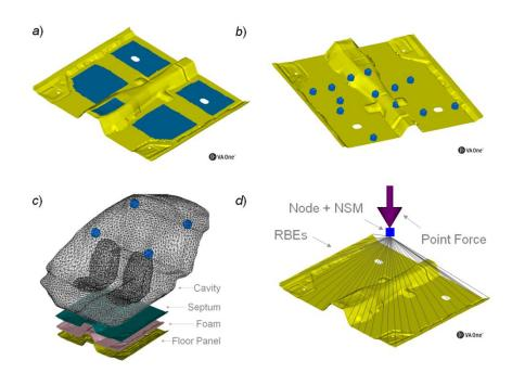
**Figure 1:** Description of model: a) Floor structure (yellow) and damping patches (blue), b) Accelerometers for average acceleration computation, c) Structure, carpet, cavity and interior microphones, d) Excitation at edge of floor panel using large mass method.
