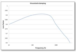
Figure 2: Aluminium-Butyl damping patches equivalent damping spectrum
