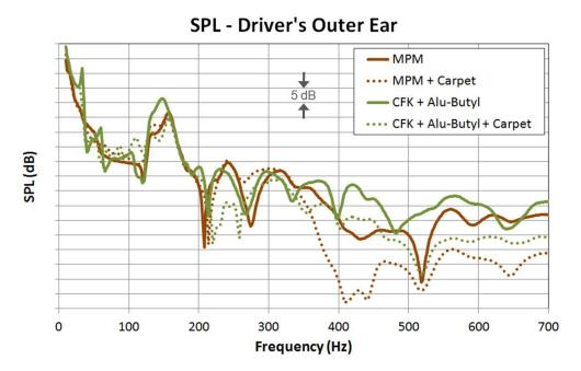
Figure 12: Effect on SPL at driver's ear of carpet on MPM and CFRP
