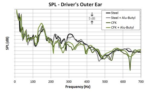
Figure 8: Effect of damping patches on car floor panels' driver's ear SPL
